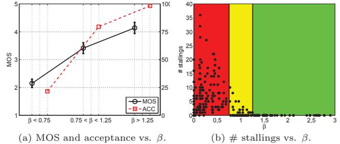
Figure 2:  $\beta = ADT/VBR$  as a KPI reflecting user experience. Users have a much better experience when  $\beta > 1.25$  – no stalling events. We refer to this + 25% over-provisioning as the  $\beta$  rule.
