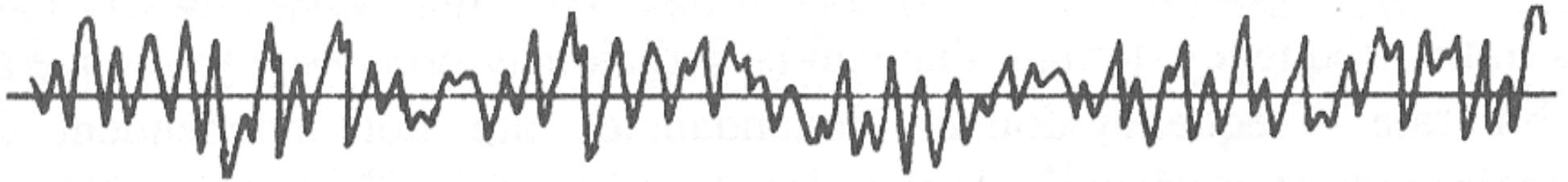
Figure 3.24 Time waveform of unvoiced sound.
